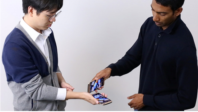
Figure 13: Tracko enables devices to support new interaction techniques, here pouring objects from one device into another.
