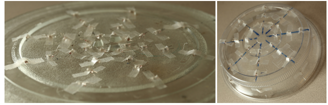
Figure 4: A turntable with 32 neon lights (left) and a plate cover with 32 neon lights (right).
